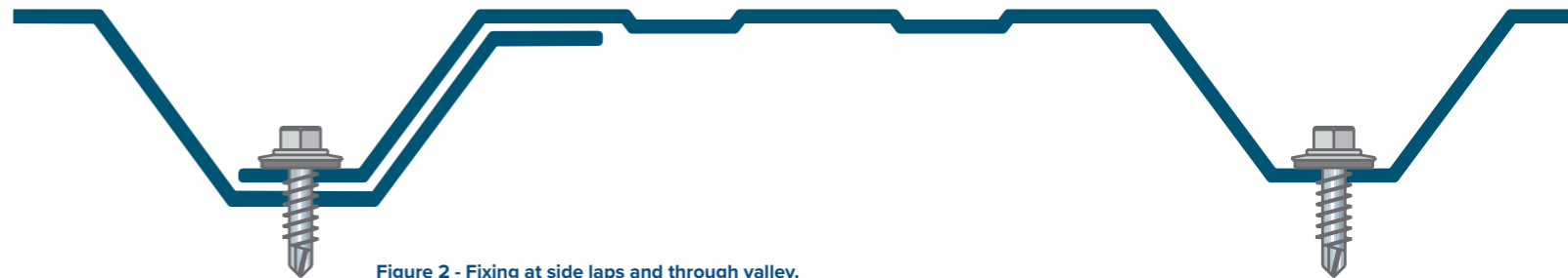
Figure 2 - Fixing at side laps and through valley.
